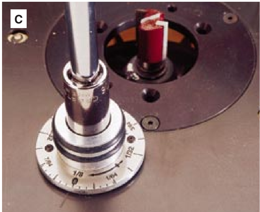
O-rings inside the Bench Dog fine-adjustment scale hold the socket shaft firmly, yet allow you to zero the scale to the index mark on the insert plate.
