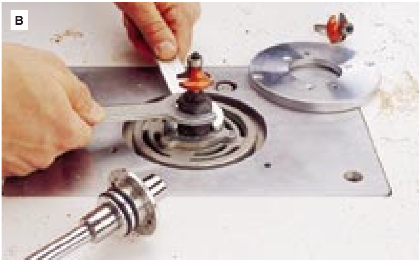
Cranking the BenchDog ProLift Ni28 to full height makes bit changing easy from above the table.
