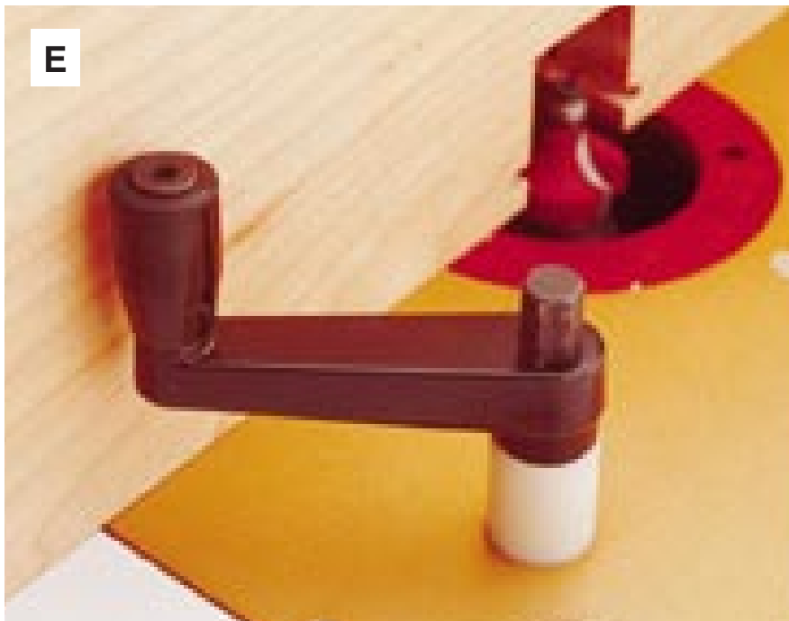
PRL's crank handle extends past the bit opening's center line and bumps the fence.
