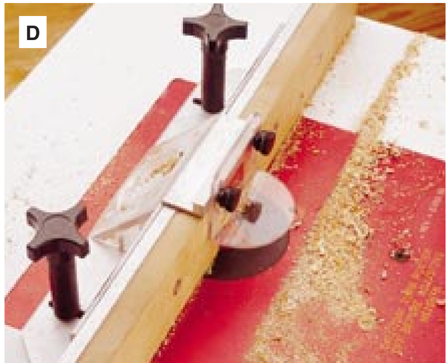
XACTA-Lift's fence features movable medium-density fiberboard (MDF) faces, a bit guard, and dust-collection port.
