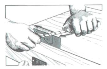
d) Hold the burnisher or screwdriver shaft at about an 85-degree angle and draww it lightly, both down and along the edge of the scraper at the same time, until a slightly even burr forms.
