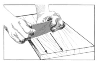
d) Hold the scraper diagonally, but move parallel to the grain of the wood.
