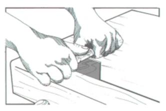
b) Remove file marks with a Medium India stone; complete honing with a Hard Arkansas stone. Avoid rocking the stones at all times.
