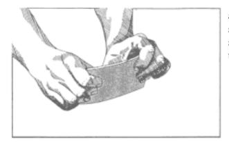
b) Angle the scraper away from you at about 70degrees from the work surface and push...
