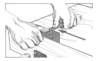
a) Clamp scraper in vise, hold file even with the blade edge, perpendicular to scraper face. Draw in long even strokes. b) Remove file marks with a Medium India stone; complete honing with a Hard Arkansas stone. Avoid rocking the stones at all times.
