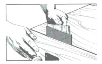
c) Move sharpening stone along both faces of the scraper until burr is completely removed. d) Hold the burnisher or screwdriver shaft at about an 85-degree angle and draww it lightly, both down and along the edge of the scraper at the same time, until a slightly even burr forms.
