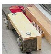
The unique feature on these bases is a switch that lets you "turn" the magnetic field on or off. Once the featherboard is in position, you simply flip on both switches to secure it to the saw table. To reposition (or remove) the featherboard, just turn the switches off.
