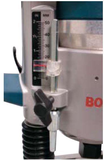
The depth-of-cut cursor on the Bosch plunge-base is extremely easy to read and adjust.
