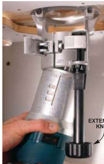
An accessory fixed base ($60) is designed for router-table use, with extra-long screws and an extension knob for easier adjustments to cutting depth.
