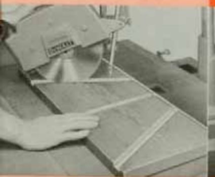
PARALLEL LEFT HAND DADO. Swivel the motor 180°, swing arm to desired angle. Mark your guide fence and make successive cuts the exact distance apart.
