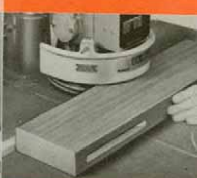
BLIND MORTISING. A fast and effective way to make a groove into which a tenon can be fitted and locked.
