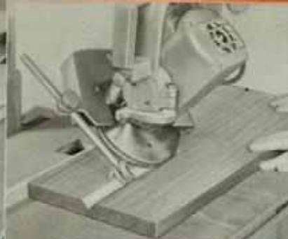
BEVEL PLOUGH. The perfect way to make "V" cuts to any depth. Your rip-scale measures for you when making a number of these cuts.
