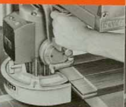
DOUBLE TENONING. A spacer collar, used in dado head, allows you to make single or double tenons with one pass across the end of your material.
