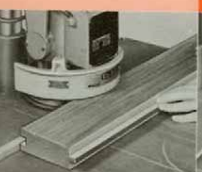
TONGUE AND GROOVE. Make your own flooring, wood panels, etc., simply by using dado inserts with collars to exact dimension needed.
