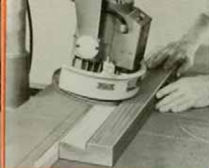
BEVEL RABBET-CUT. Simply tilt the motor and you can make any desired angle cut in your rabbeting operation.
