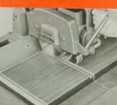
CUT OFF AND DADO. Saw blade and dado head combine to give you this unusually fast, accurate job in a single operation.
