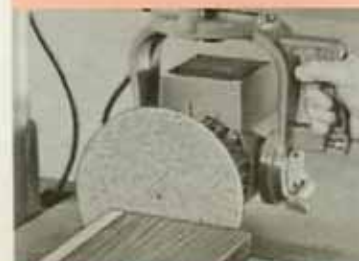
BUTT SANDING. Made easy across the end of the stock or at any miter, bevel or double angle desired.
