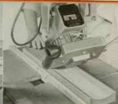
RADIUS CUTTING. Tilt dado, and push work through as in ripping—and you get a fine concave cut full length of the board.
