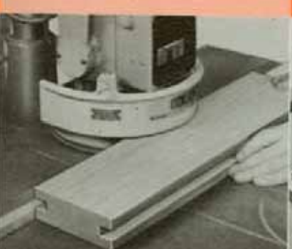
GROOVING. Dado Head gives you extra-wide groove cuts, eliminating a number of passes when made with saw blade alone.
