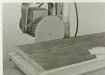
STRAIGHT EDGE SANDING. Set disc sander parallel and along the guide fence. Push stock past for straight edge work.
