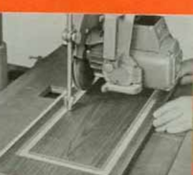
PANEL SINKING. Lower the dado 1/8 inch and make cuts illustrated by pushing stock. You can easily square corners with hand chisel.
