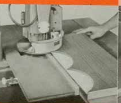
SCALLOPING. Feed the stock against the dado as shown and put unusual scallop design on your window valances.
