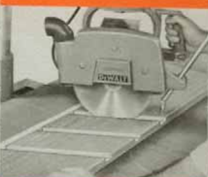
ANGLE DADO. A special cut which finds many uses, accomplished similar to mitering with saw!
