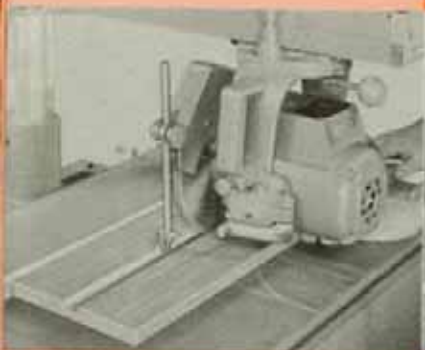
PLOUGHING. Cutting a set depth and width, full length of stock with great accuracy is a big feature on the DEWALT Power Shop!
