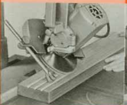
FLUTING. Simply a series of parallel "V" grooves, for decoration. Used to simulate pillars or columns in cupboards or fireplace mantels.
