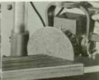
MITER SANDING. Set material on special table. Swing arm to desired miter angle. Pull sander disc across stock for smooth, perfect cuts.
