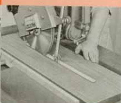
CENTER PLOUGHING. This cut is made by lowering dado into your material and raising it at the end of cut.
