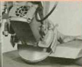
DOUBLE MITER SANDING. Swing arm to desired angle. You are all set for compound sanding work. Pull disc across precut stock.
