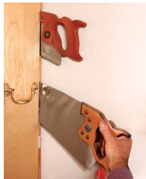
Storage behind the cabinet. A carpenter's square on one side and three panel saws on the other fit into slots in the back of the cabinet.
