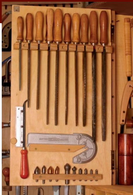
Hinged panels add storage. Tools hang on both sides, adding 40% to the cabinet's hanging area.
