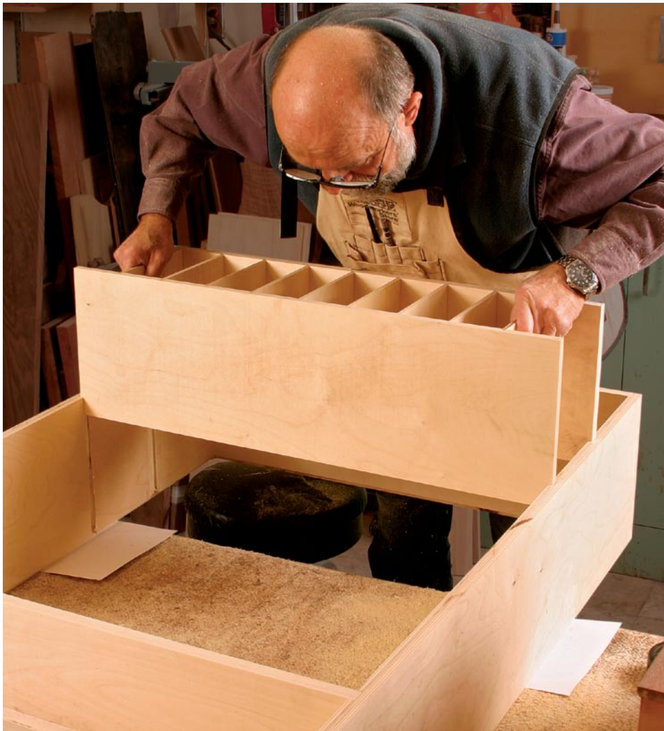
Install the upper shelf and gallery. Cut a dado on both sides of the cabinet and install the upper shelf. This gives the carcass extra rigidity. After routing the dados for the upper and lower shelves, test-fit the gallery and then glue it in.
