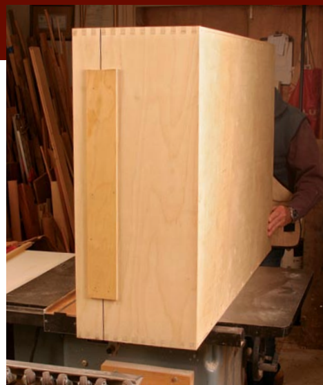
Cut away the door section. With the front and rear panels installed, cut away the front quarter of the box to form the main doors. Cut the short sides first, and then tack a batten across the cut to hold the section in place while cutting the long sides.
