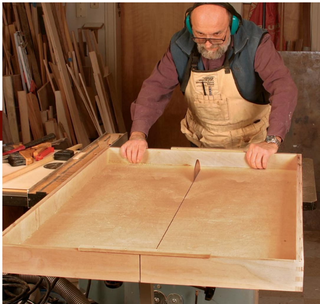
Next cut makes the two main doors. Tack two strips of wood across the cut line as shown. Then set the sawblade to just score the underside of the strips. In this way the panel is cut in half but won't bind on the sawblade.
