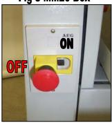
Fig 9 On Off Switch
