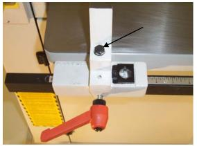
Blade drift means the blade isn't cutting parallel to the fence. Every blade will cut in a slightly different manner and you may have to adjust the fence angle to compensate for this drift. To check blade drift, mark a straight line on a board 24" long, rip the board freehand while carefully following the line About halfway, through the cut, stop the saw and leave the board in place. Mark the side of the board on the saw table with a soft pencil. This line indicates the
