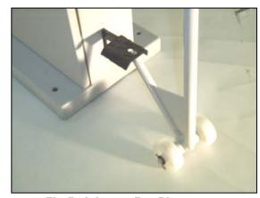
Fig 5 Johnson Bar Placement
