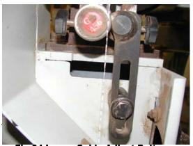
Fig 24 Lower Guide Adjust Bolt
