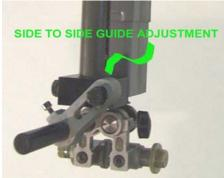
Fig 15 Horizontal Adjustment
