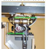
bracket. Align the guides and tighten the allen screws. Back the guides off and then move them back together to double check the adjustment before re-installing the
