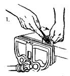
To Sharpen a Bevel Edge Scraper Blade remove the old burr with a smooth mill file held flat against the face or flat side of the blade.
