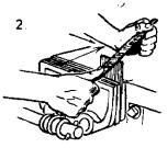
File or grind a bevel of about 45°. Push the file forward and to the side with one sliding motion.
