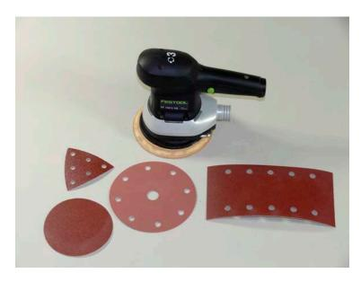
Random orbit machines rotate a pivot point while allowing the attached but not mechanically driven pad to move
