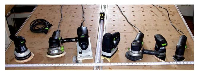
There are basically three different ways the abrasive can be moved by a machine sander: *linearly in a fore-aft motion, in a circle in a rotary motion, or back and forth in an arc.* Festool uses the first two motions but not the arc motion.
