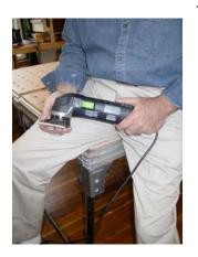
you constantly move the machine, the same sanding grit passes the surface of the work piece at the same location repeatedly leaving often hard to remove deep scratches. The DX sander does not do this
