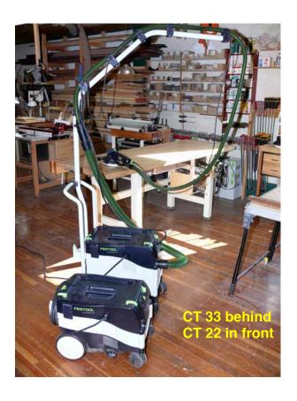
gets taller. A CT 22 is shown in front of a CT 33 in the photo on the previous page. Notice how the white lower section is taller on the CT 33 than on the CT 22. They draw 134 CFM and pull an impressive 90" of static water lift (23000Pa) while generating only a 72dB noise level.
