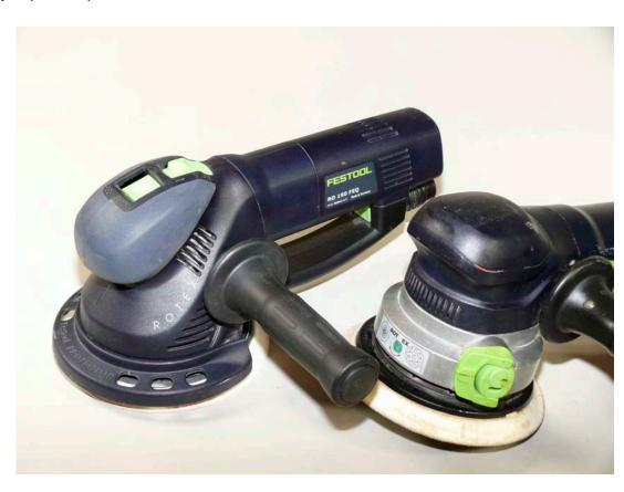
150mm (6") pad unit or the 125mm (5") unit (both shown here for size comparison), feature a switch selectable sanding
