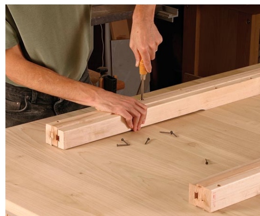
Mount the slides. Use screws to secure one end of the slide to one of the top halves (left). Then screw the opposite end of the slide to the other half (above).
