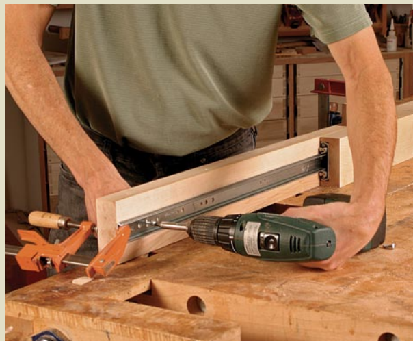
Assembling the slide. The main part of the drawer slide screws into the channel piece. Screws also are used to mount the drawer-slide leg to the extension piece (above).
