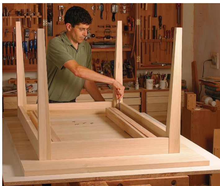
Attach the base to the top halves. With all the parts upside down, Miller mounts the table aprons to the underside of the top halves.
