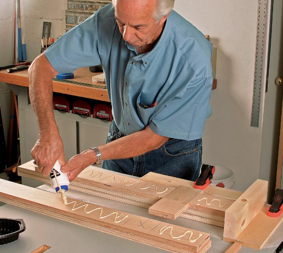
Leg assembly. Insert a taped spacer block to hold open the lower mortise. An L-shaped jig keeps the sections aligned. Use a generous amount of glue, but don't apply glue to those areas that face the spacer block.
