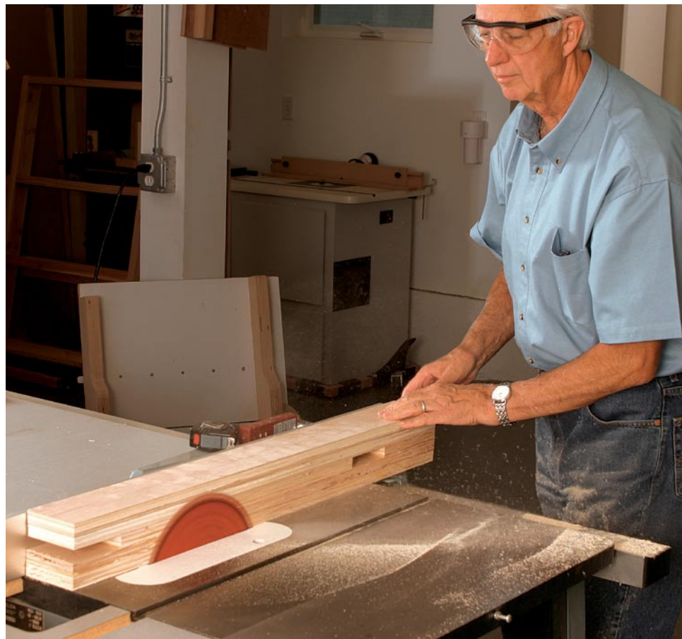
Clean up the edges. After the legs, aprons, and stretchers have been assembled, run both edges past a sawblade to clean up glue residue and leave them at the final 3½-in. width. Cut the first edges with the fence at 3⅛ in., and the opposite edges at 3½ in.
