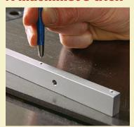
To create a tight fit in the miter slot, use a center punch to create dimples on the side of the guide bar nearest the blade. Place dimples 1/8 in, from the top of the bar, starting 1/4 in. from the ends and spaced every 3 in. File the dimples to fine-tune the fit.
