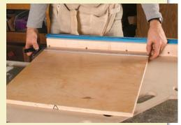
Measure the difference. Measure the width of the board adjacent to the fence and at the opposite end. If there is a difference, the fence isn't perfectly square to the blade.
