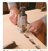
Cut out the handholds. Multiple handholds make it easier to maneuver the bulky sled on and off the saw, and also slightly reduce the weight.
