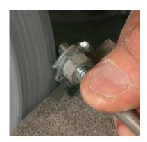
Customize the nuts for MDF. Designed to penetrate wood, the long spurs on the T-nuts need to be shortened to go into MDF. Attach a nut and a T-nut to one of the bolts used to secure the plywood fence to the
