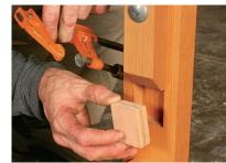
**Locking blocks.** If you are worried about the combined weight of the sled and a heavy workpiece causing the horse to shift, clamp a custom-size block into the gap below the upper stile.
