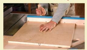
The first cut. Take a piece of plywood, about 20 in. sq., with one side perfectly straight. Place this side against the fence, mark the opposite side with a triangle, and cut one of the adjacent sides using the sled.
