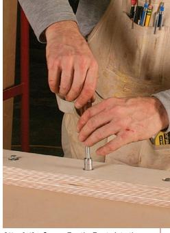
Attach the fence. Tap the T-nuts into the underside of the sled, slide ¼-in.-dia. bolts through the fence, and then use a socket wrench to drive the bolts into the T-nuts.
