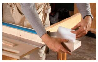
A straight fence. Clamp the two sections of fence together, and use pieces of paper as shims until a straightedge verifies that the front of the fence is perfectly straight.
