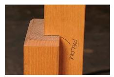
Mark its position. Once you have the sawhorse set, mark the point where the stiles meet, and where the feet are located on the floor. Now you can use the horse elsewhere and reset it quickly.
