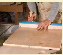
The second cut. Flip the test board 180°, keeping the same side against the fence, and cut the side opposite the first cut.
