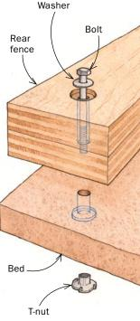
its length. To achieve this, the fence has two parts: a plywood rear section that is screwed to the bed of the sled, and a hardwood face that is added later. The rear piece gives the fence its stiffness. It consists of two layers of <sup>3</sup>/<sub>4</sub>-in.-thick Baltic-birch plywood laminated into a 1½-in.-thick by 4¼-in.-wide bar. True this up after lamination.
