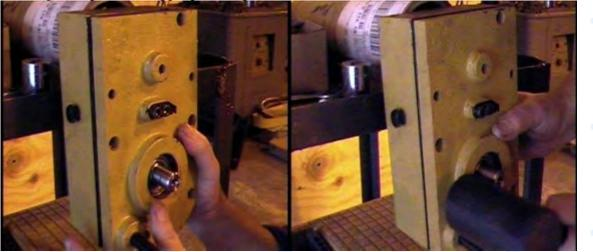
Tighten all of the screws in an alternating sequence.
