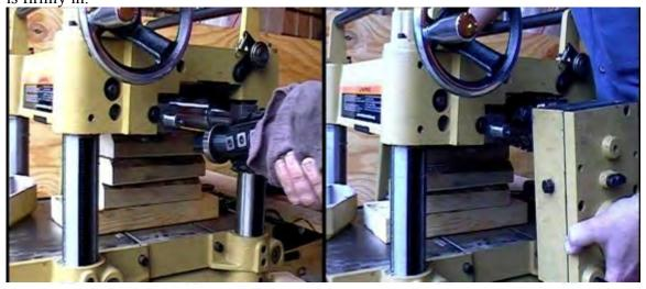
32. Tap the gearbox to seat bearing into place.
