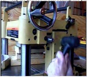
33. It may be necessary to turn the handle in order to align and start the bolts, then tighten them.
