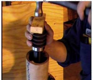
25. Installing the head in the gearbox by pressing it in the new bearing. Reinstall the oil seal.
