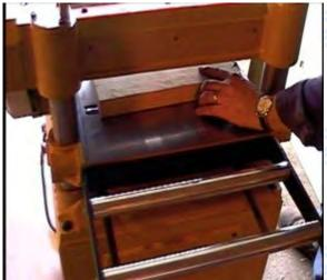
Loosen four bolts holding the gear box.
