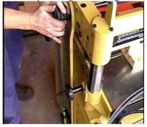
2. Remove pulley bolt, rotate the cutterhead until the key is in the upright position, then remove the pulley and key.
