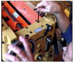
34. Reinstall the keys and gear/chain assembly, Tension roller spring, side cover, and the handle with it's key.
