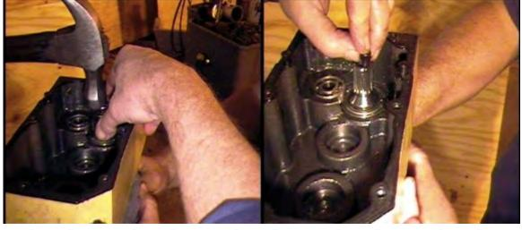
27. Reinstall the washer, screw, helical gear, and bolt.
