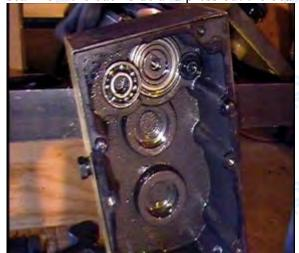
24. At this time, install the bearing on the pulley end of the new head (snug press fit). The pulley can be use to seat the bearing. With the outside of the pulley (large OD) against the bearing, tap it into place.
