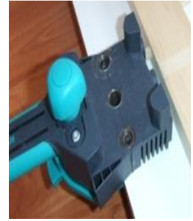
Drilling template: used to correct centering holes on the edge of the plate and alignment holes on two different boards.
