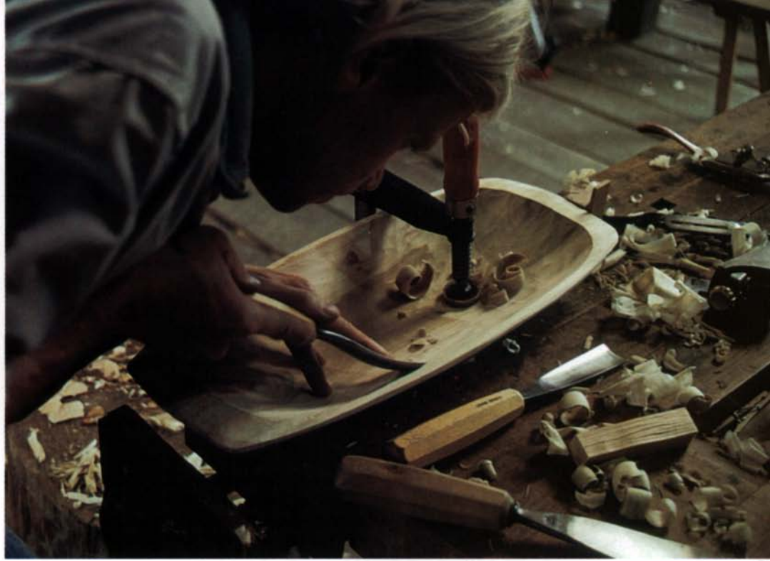
Above: After shaping the rim, taper the outside ends of the bowl, first chopping off the corners of the blank and then the remaining wood until the outside shape parallels the inside. Right: Fine-tune the width of the rim as you smooth the inside gouge marks with a wider, flatter gouge.
