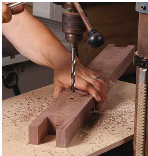
Pegs are a design detail. Locate and drill holes in the posts (left). Dry-fit the feet, stretcher, and posts, and use a brad-point bit to mark the peg location in the stretcher (right). Disassemble and drill the stretcher.
