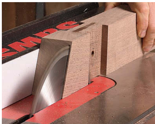
Angle and thin the end of the stretchers. After cutting the angle on each end of the stretcher on the miter saw, use the table saw to trim the block beyond the half lap. With the blade fully raised, rip in and back out (left). Snap off the thin waste (right) and clean up with a block plane.
