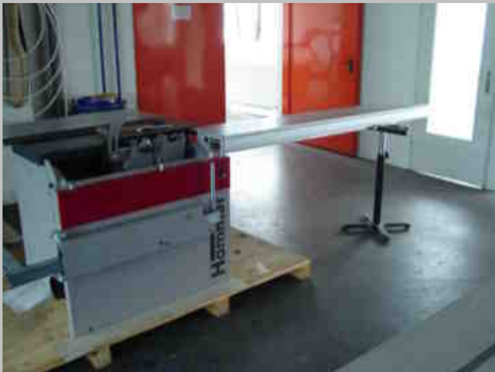
Figure ST01.1 Sliding table in place ready to be slotted over the securing screws
