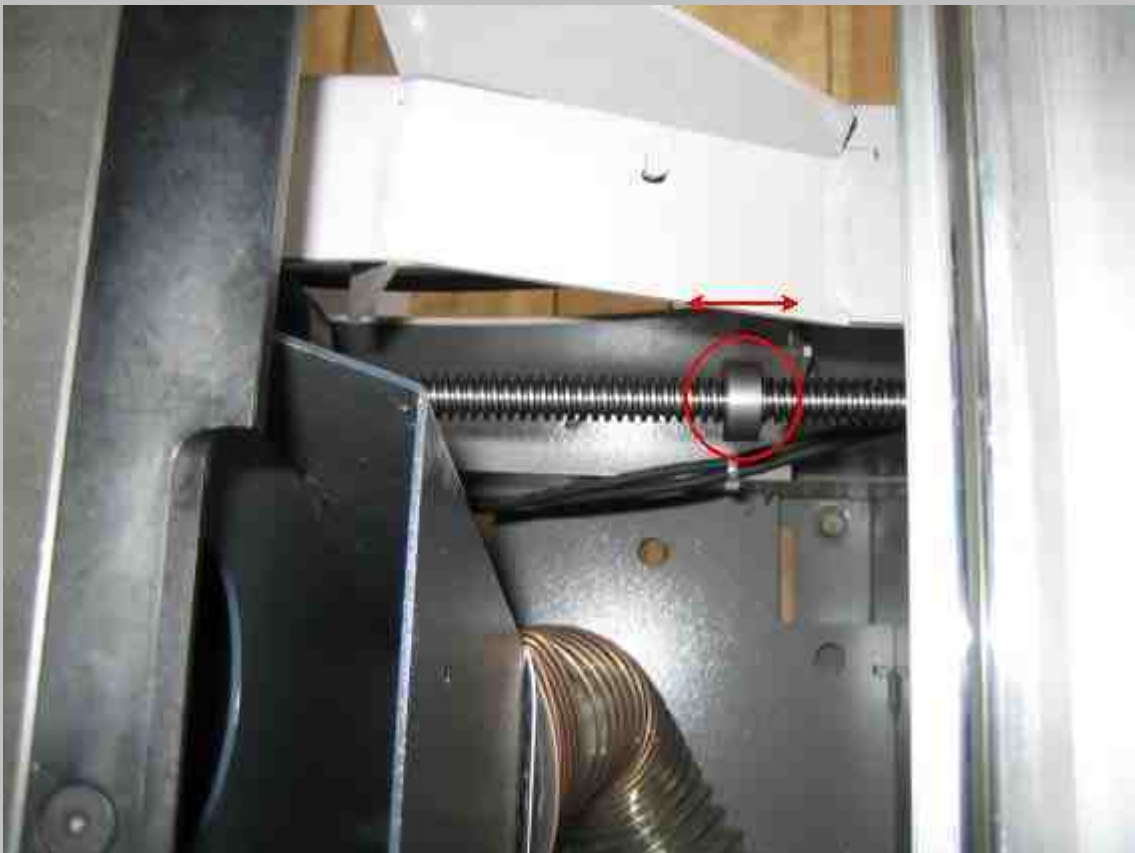
Figure SR08.1 Showing the 45° Mechanical Stop
