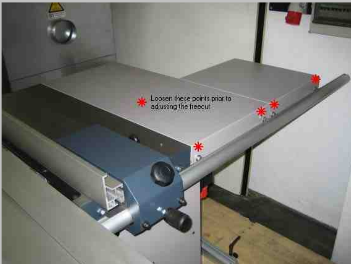
Figure SR04.4 Rip fence bar securing points
