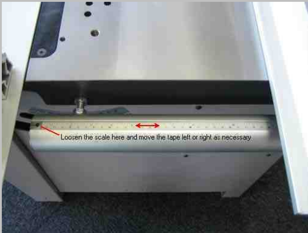
Figure SR09.1 Scale adjustment on the Guide bar
