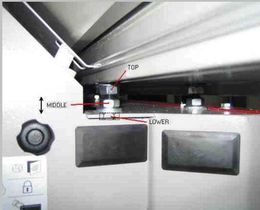
Figure ST01.6 Showing the three locking nuts. ONLY use the top one to lock the sliding table in place!
