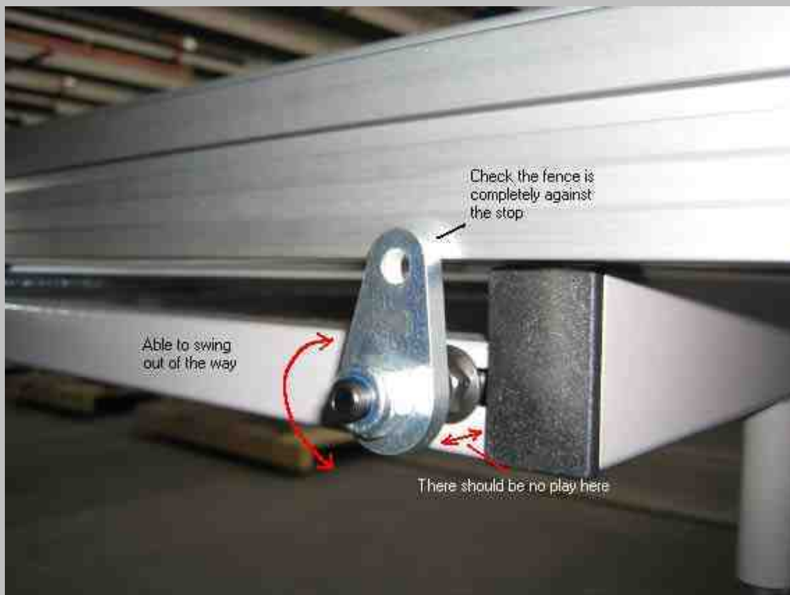
Figure SS05.2 Crosscut fence 90° adjustment
