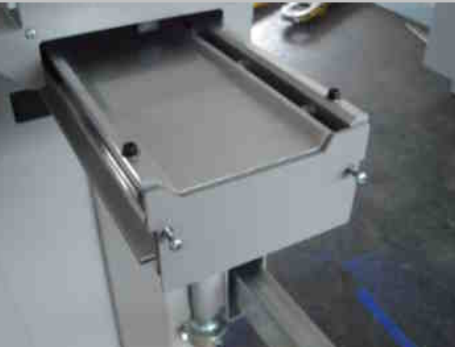
ST01.7 Coverplates for sliding table bed
