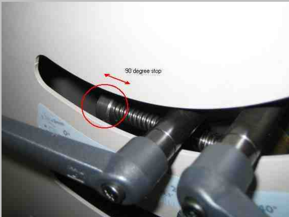
Figure SH02.1 The 90° stop on the tilt-controlling axle
