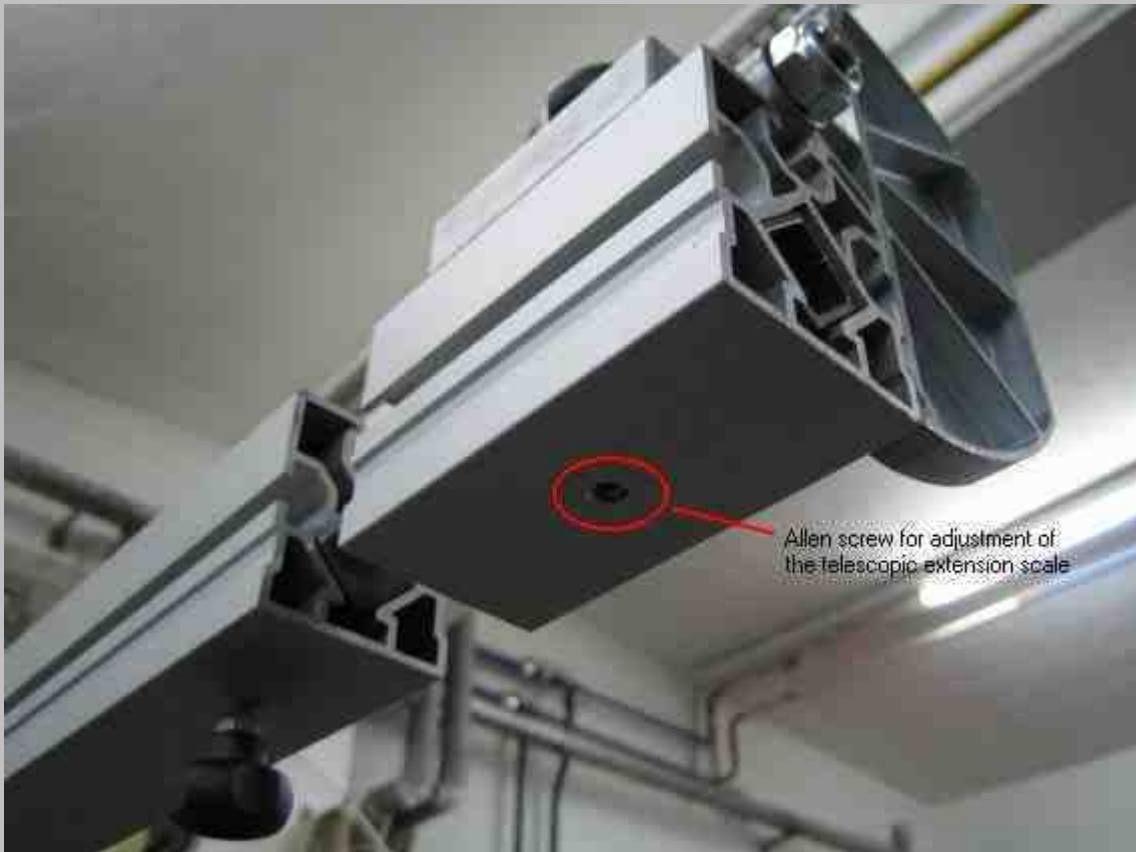
Figure SS07.3 Crosscut stop and block adjustment
