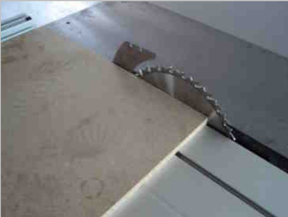
FC01.1 Checking freecut on the sliding table
