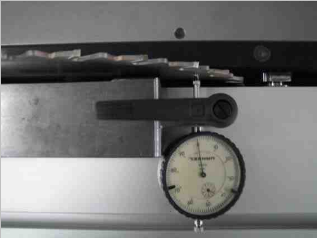
Figure SS01.1 Start position of the dial indicator
