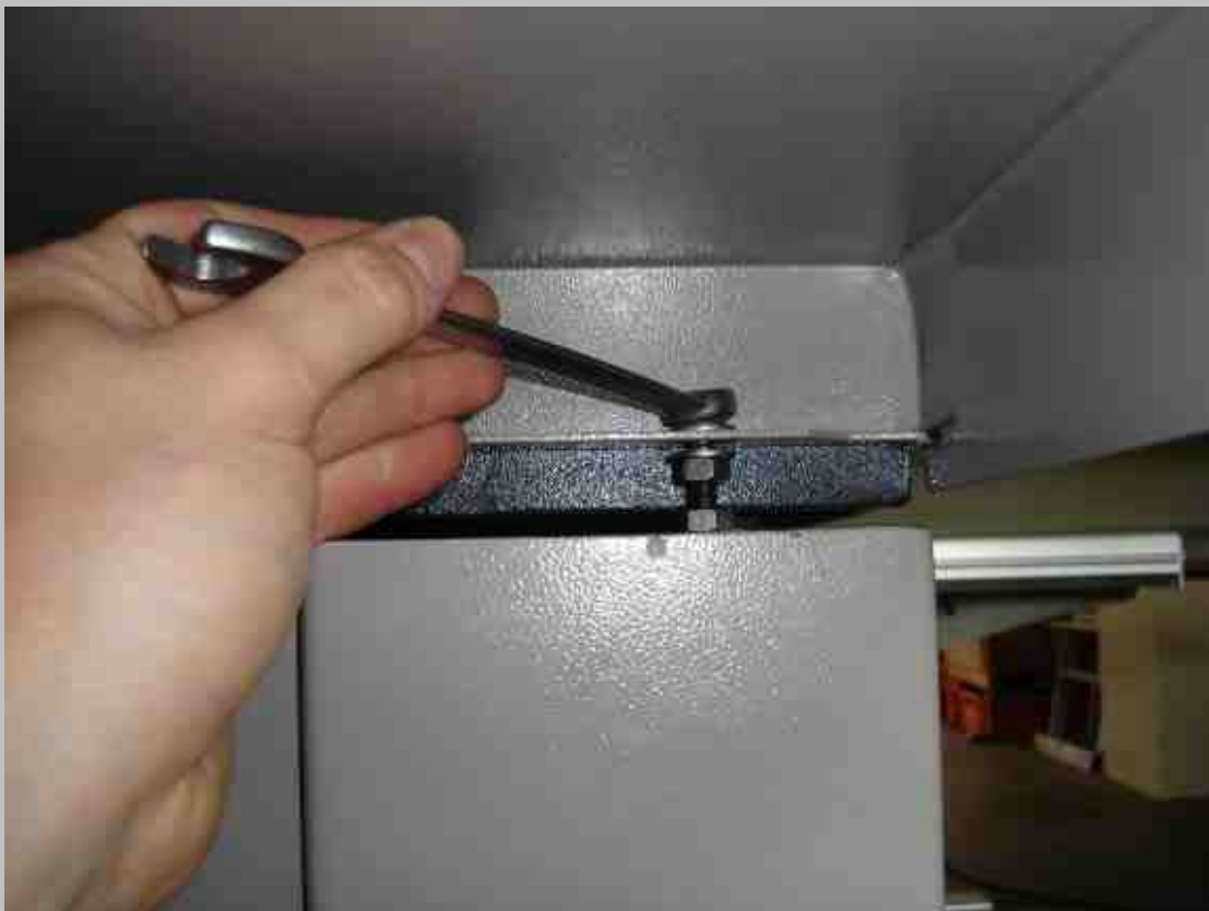
(Adjusting the table to match the height of the cast iron table)
