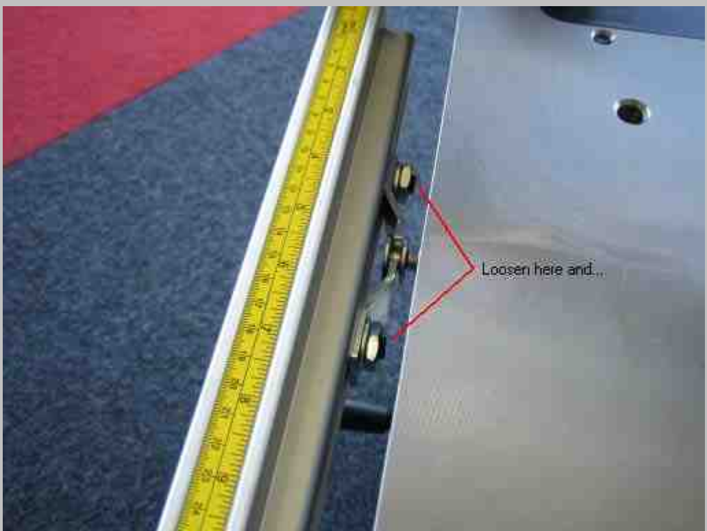
Figure SR09.2 Combination machine scale adjustment
