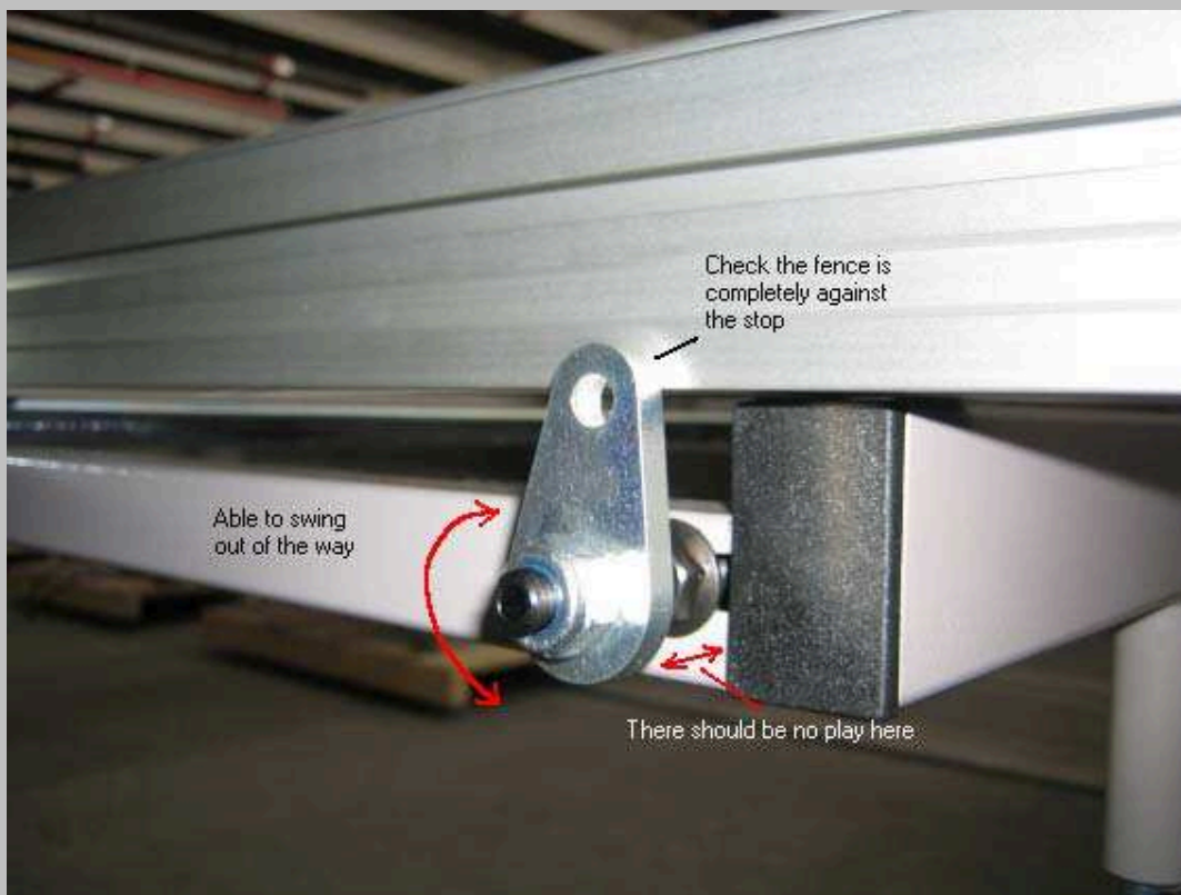
Figure SS05.2 Crosscut fence 90° adjustment
