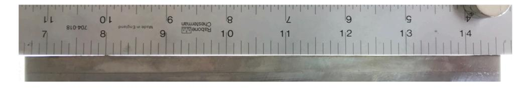
After carful sharpening with Makita 9820-2. Light gap of 0.001 inch measured with feeler gauge.
