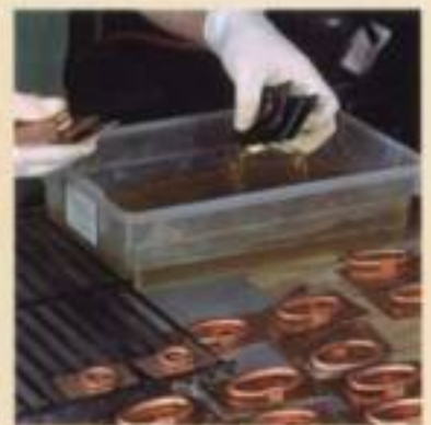
A fast patina. To give the pieces a seasoned look, hardware is dipped in a mixture of natural extracts, then heated with a blowtorch.
