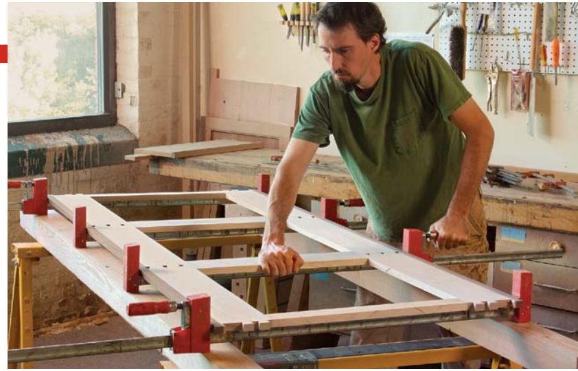
Create two frames. The two lower stretchers are connected by the drawer runners. The two upper stretchers are connected by the kickers.
