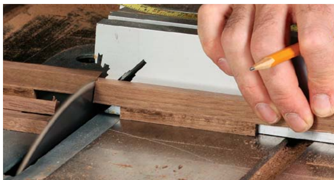
Rip tricks. The first two rip cuts form the tenon (left). Leaving the angled cheek cut for last lets the handle stock fall away from the blade (right).
