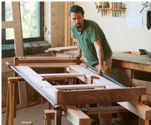
Add the lower frame to the legs. One long clamp on each side is enough to pull it all together.
