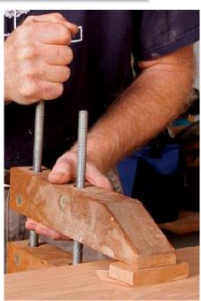
**Glue and clamp.** After dry-fitting the patch (it should fit evenly and be slightly proud), glue it and clamp it in place with plenty of pressure. Waxed paper prevents the caul from sticking to any squeeze-out.
