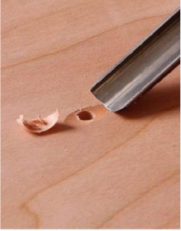
**Scoop around the hole.** Take a deep carving gouge that is slightly wider than the damage, in this case #8/10mm, and carve out a shallow depression around the hole. Practice on some scrap first.
