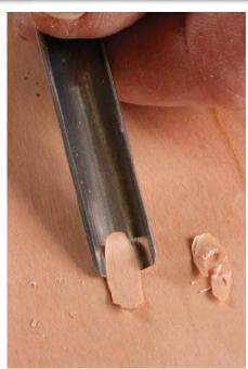
**Create a patch.** Place the piece you just removed on a piece of scrapwood that closely matches it in grain and color. On a tabletop, your best bet is the underside. Using the same gouge, scoop out a slightly deeper patch.
