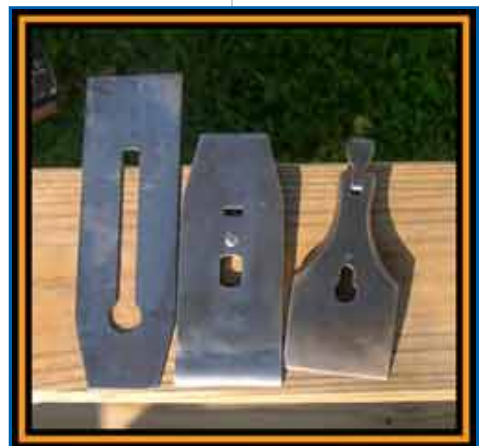
Hole is still at top not bottom, patent date on cap iron (chip breaker)
