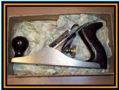
Parallel knurling on the brass depth adjuster is back
