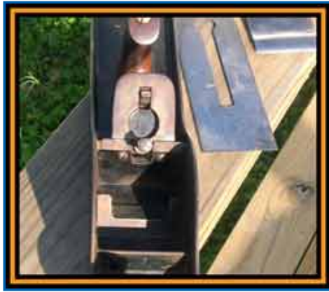
All New Frog Design, The mouth opening is Non-Adjustable and fixed
