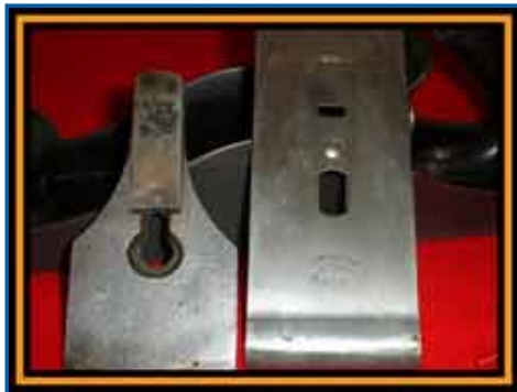
Lever cap spring is now rectangular.
