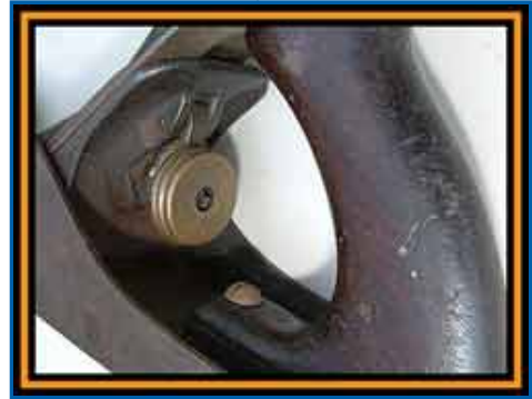
Ballon Shaped Knob with Bead at Base
