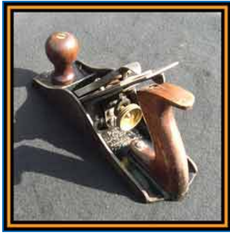
First Year Larger Brass Depth Adjuster Knob
