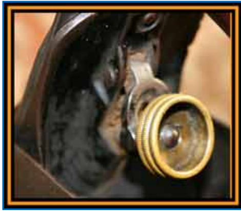
The brass adjusting nut now has a left-hand thread.
