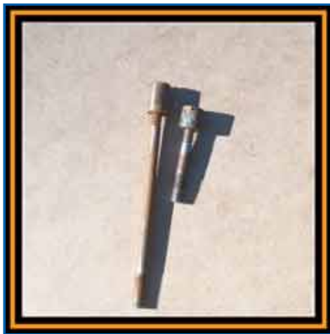
Read Nut on Handle Studs is Longer than Front
