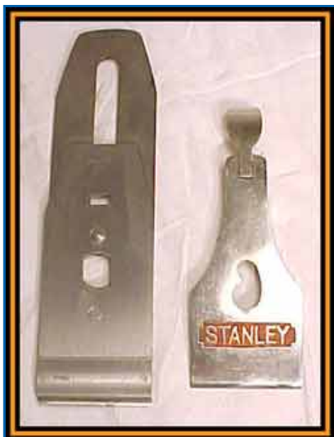
Rounded top on plane iron
