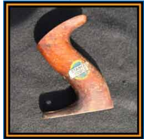
Decals on totes are most common on Type14s You also see some on late T13s and early T15s
