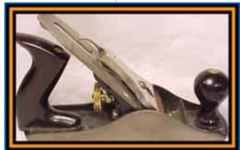
Rounded shape to top of rear handle
