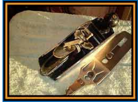
New Diagonal Knurling on Dept Adjuster
