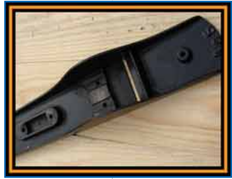
Frog receiver has two shallow grooves, parallel to the plane's sides, cast into it. The screw holes are located in the grooves. You can't see in this image
