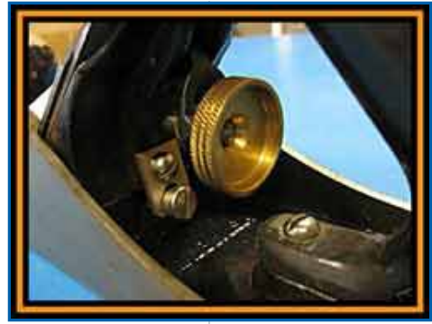
New Diagonal Knurling on Dept Adjuster
