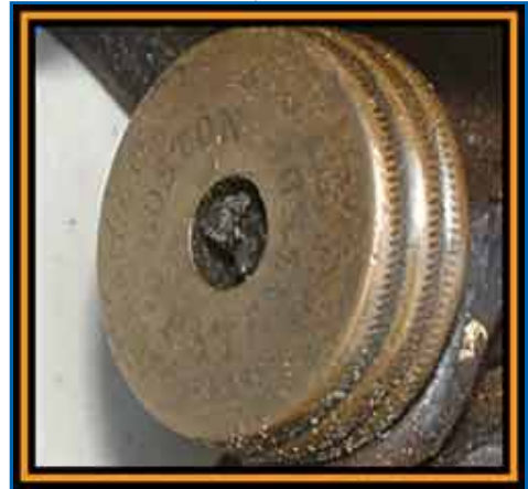
Solid Brass Depth Adjusting Nut (sometimes of a two-piece construction), with "BAILEY, WOODS & CO." "BOSTON" "PATENTED" "AUG. 31, 1858, AUG. 6, 1867"
