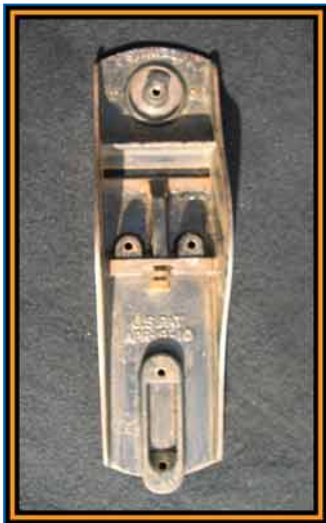
New Raised Ring cast into bed where knob base sits to stop splitting of knob..
