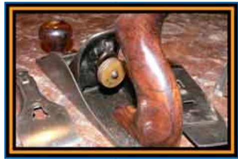
Earliest models do not have Bailey's name, nor Boston, on the brass adjusting nut.
