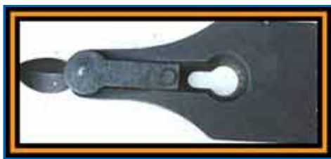
The back of the lever cap is solid and has a Banjo-Shaped Spring..
