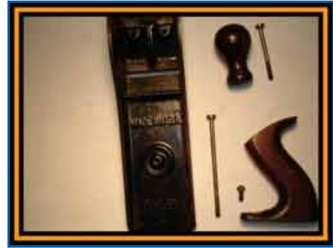
All Steel Handle Screws with out a brass Nut due to WWII Brass Shortage
