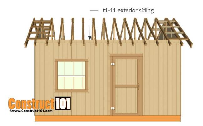
Cut t1-11 siding to size and install between the rafters. Use 1 1/4" finishing nails to install.
