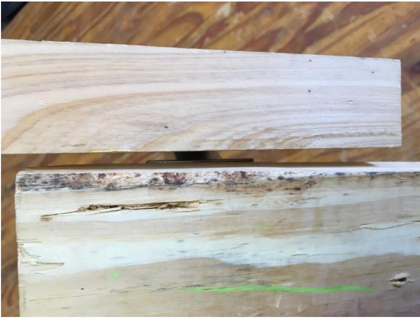
Revel is at 0.25" (Stile on top – frame on bottom)
