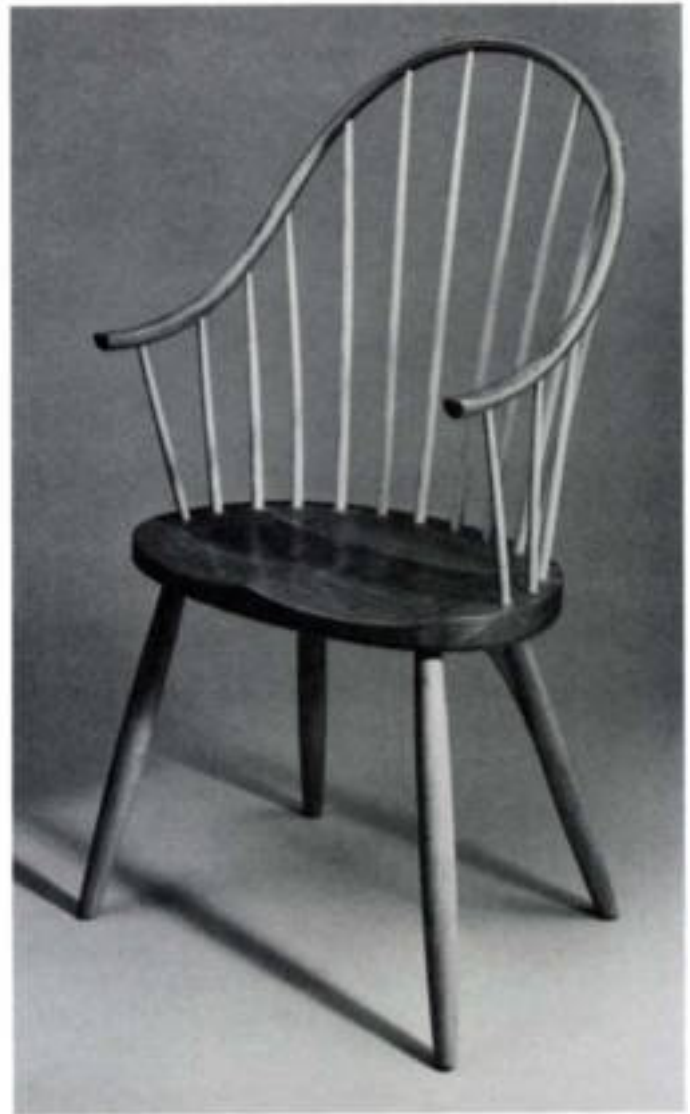
Continuous-arm Windsor chair, made by Thomas Moser of New Gloucester, Maine. Overall width: 22\frac{3}{8} in. Overall height: 41\frac{3}{4} in. Seat height: 17\frac{1}{2} in. Seat pitch: 2^\circ . Back pitch: 12^\circ (at two center spindles). Seat depth: 15\frac{1}{8} in., 14\frac{1}{8} in. usable. Seat width: 22\frac{1}{4} in. Height of arms above seat: 10 in. Weight: 11\frac{3}{4} lb. Price: $295.
