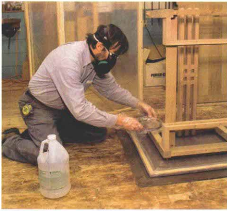
Aqueous ammonia is poured into a glass container placed at the bottom of the fuming chamber (above). Then the top of the chamber is lowered quickly onto its base (right). Protective gear is essential.
