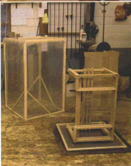
Fuming with ammonia gives white oak that classic golden-brown color. Before it's been fumed (inset), white oak is a pale, almost cool, tan.
