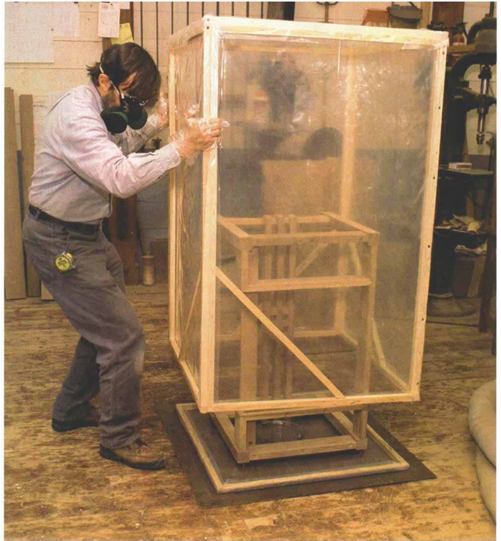
Aqueous ammonia is poured into a glass container placed at the bottom of the fuming chamber (above). Then the top of the chamber is lowered quickly onto its base (right). Protective gear is essential.
