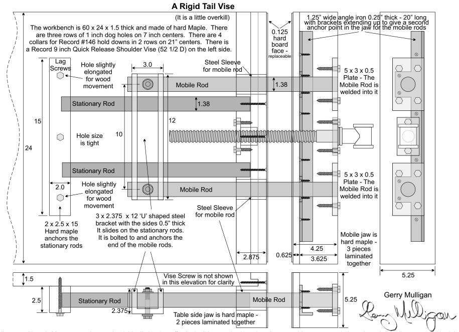
When I built my workbench 38 years ago I wanted a rigid tail vice that effectively did not rack when clamping something at one end. I purchased a quality screw and had the other components fabricated from my design by a local metal shop. I saw a design which I modified, but I have not been able to relocate that reference, or even other examples. So, a sliding bracket on a set of stationary rods is not original to me, but I don't know who to give the credit to.
