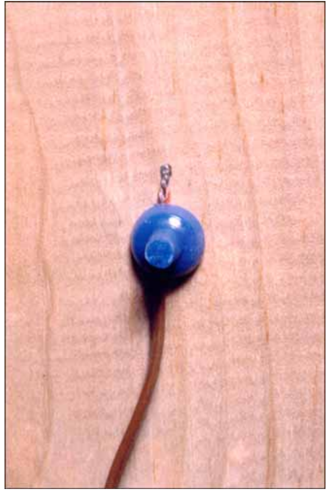
Figure 2—Surface thermocouple held in place by push pin.
